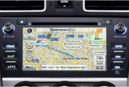
74 OE navigation with DAB (LHD/RHD) 86271FJ490/86271FJ370 Access internet radio and more with the SUBARU STARLINK* 3 infotainment system. Control it with the 7-inch touchscreen, steering wheel controls or voice recognition* 4 . Use your iPhone* 1 or other mobile music device via the USB or AUX jack. *Requires GPS antenna.
