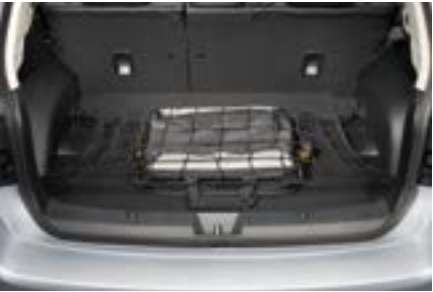
63 Cargo Net (Floor) F5510FJ100 Helps prevent the cargo/luggage from shifting when the vehicle is in motion.
