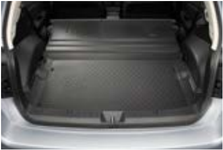
62 Foldable Cargo Tray J515EFJ100 Protects cargo area floor from dust and dirt. Also offers extra protection when the rear seats are folded flat.
