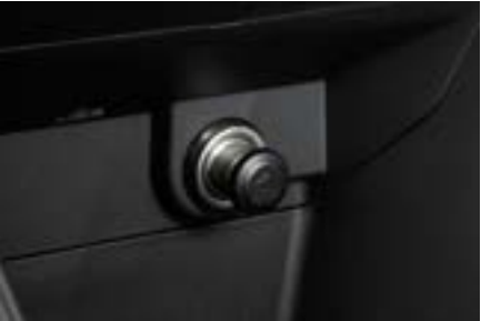
56 Cigarette Lighter Kit H6710FJ000 Installs into the accessory socket location in the covered centre console pocket.
