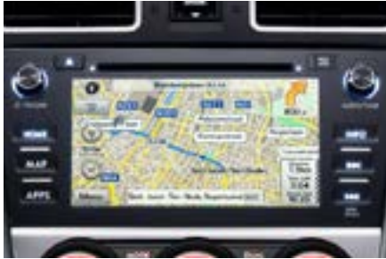
73 OE navigation without DAB (LHD/RHD) 86271FJ470/86271FJ360 Access internet radio and more with the SUBARU STARLINK**3 infotainment system. Control it with the 7-inch touchscreen, steering wheel controls or voice recognition**4. Use your iPhone**1 or other mobile music device via the USB or AUX jack. *Requires GPS antenna.
