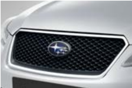
1 Front Grille J1010FJ050 Produced with a mesh finish that creates a fresh new facial image.
