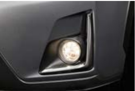
6 Fog lamp & DRL kit H4510VA020 Enhance vision in inclement weather.
