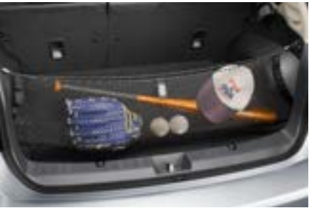
66 Cargo Net (Rear) F551SFJ100 For a clean and tidy luggage room. Stretches across the cargo area to hold various types of luggage.
